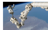
'Canadarm', mechanical arm used on the Space Shuttle Image Author: NASA Image Source: http://en.wikipedia.org/wiki/ File:Sts114_033.jpg
